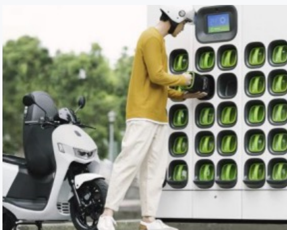
Figure 27. Example of battery swapping station for e-mopeds
