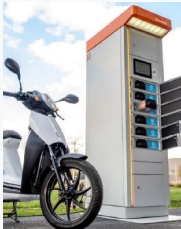
Figure 29. Gogoro moped and battery swapping station
