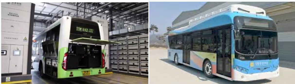
Figure 30. E-bus with swappable batteries in China (left) and South Korea (right)
